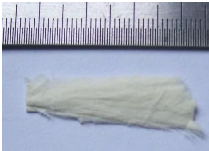
Appearance of boron nitride nanofibers
