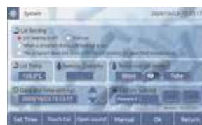
Setting interface Hot lid temperature and working mode of hot lid can be set
