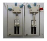
Small & Big Syringe Pump Assembly 25μL(left) and 1000μL(right) syringes capable of dispensing 1μL-1000μL volumes.
