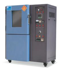
Air–ventilation aging test chamber is suitable for heat resistance test of electrical insulating materials, electronic spare parts, gas aging test of plasticized products, to check its adaptability to storage and operation under high temperature environment conditions, compare the properties after aging in air under simulated high temperature and atmospheric pressure. This product meets JB / T7444 "air heat aging test chamber" and GB / T3512–2001 test standard requirements.
